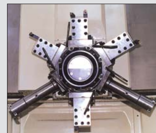
Electrical V-6 Turret(VTB-100T only)
