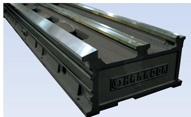
The extra wide (1150mm) one-piece solid bed of Meehanite cast iron construction is densely ribbed to withstand the brutal forces of heavy cutting and loading. This extremely rigid bed is fully stress relieved, induction hardened, and then precision ground in one set up for inherent accuracy.
