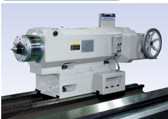
The heavy duty box type tailstock of high quality cast iron construction boasts a large 270mm diameter quill and a built-in rotating spindle. The tailstock is designed to handle workpieces of up to 12 tons pounds between centers without steady rest.
